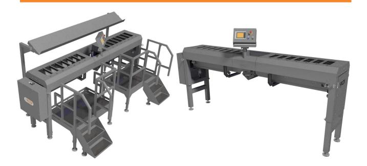
**Thor** is a combination weigher with manual loading, suitable to compose doses according to a prearranged weight (never lower). Produces are positioned by operators directly on the scale/hoppers, then the Thor calculates the best combination of available weights to compose the dose. Produces fall on 2 soft wave belts and are outfed on a central hopper.
